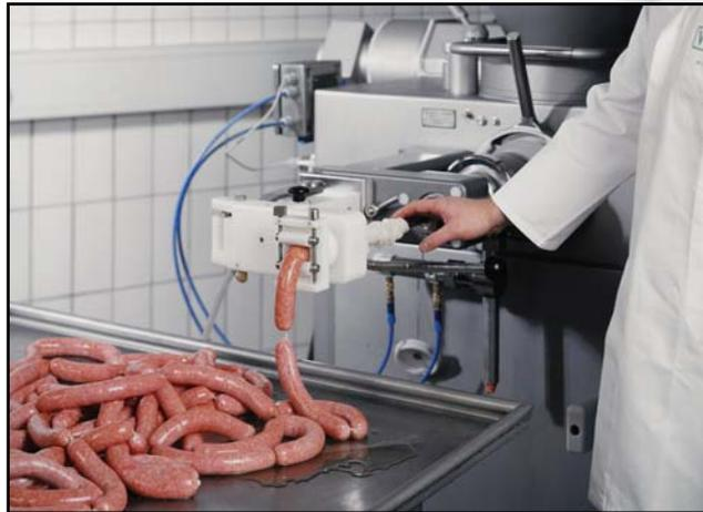
ROBOT HP15C with sausage grinder 980 and automatic separation valve
